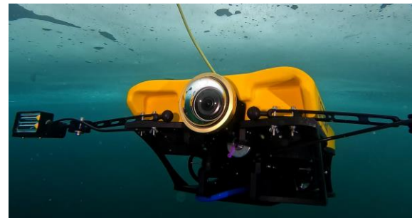
Vision sensor embedded ROV
