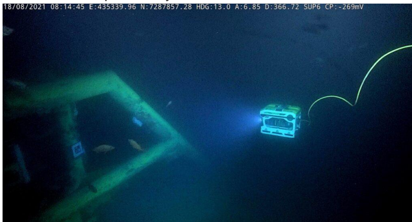
Wind farm inspection by ROV
